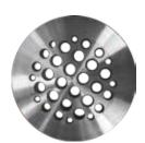
Flanged assembly consisting of a series of orifice plates to produce a specified reduction in line pressure or to create a critical flow, giving controlled flow rate regardless of changes in downstream conditions. In-house expertise covers all aspects of design and manufacture associate with restriction of pressure for control purposes.
